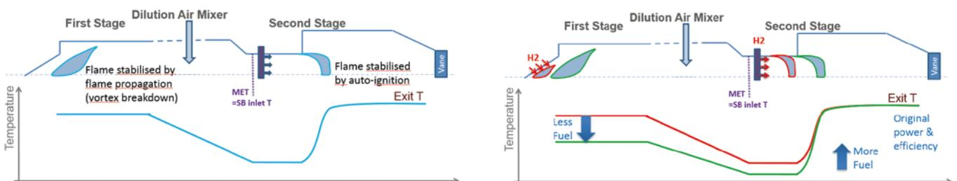
1 | Schematic of sequential combustion with flame positions for natural gas (left) and hydrogen (right).
