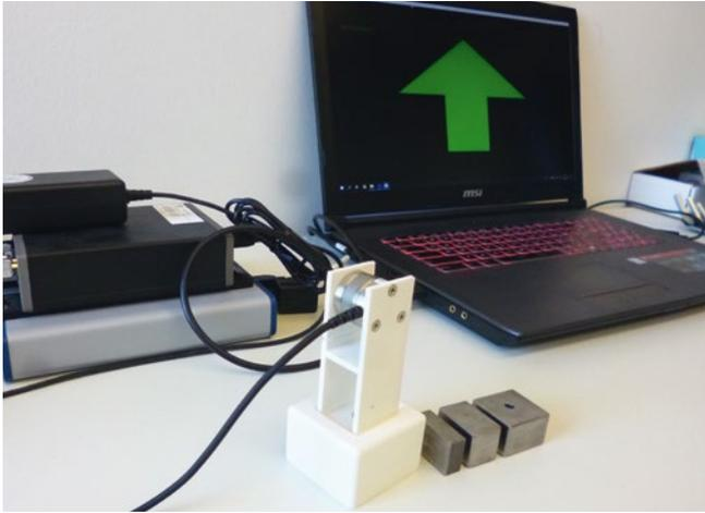
1 | Experimental setup for the object manipulation task for the human participants. Object is printed with a 3D printer and force transducer (Nano 25, ATI) mounted in the middle of the object. Subject will pick up the object with 4 different weights and hold for 5 seconds. The grip force is measured with 1kHz sampling, and compared for different materials applied on the subject's finger tips in order to investigate the effect.
