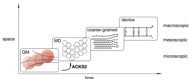
1 | Illustration of a multiscale approach in material modeling. The ACKS2 model provides efficient quantum-mechanics level derived electronic polarization for force field simulations.
