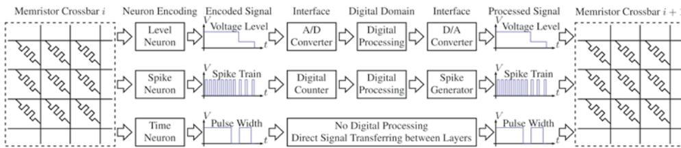
2 | Hardware implementation of neuromorphic computing with three different encoding mechanisms.
