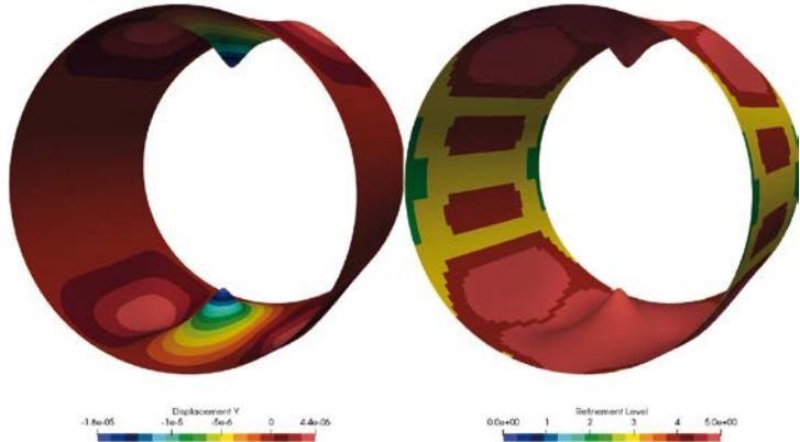
2 | Displacement of a pinched cylinder.
