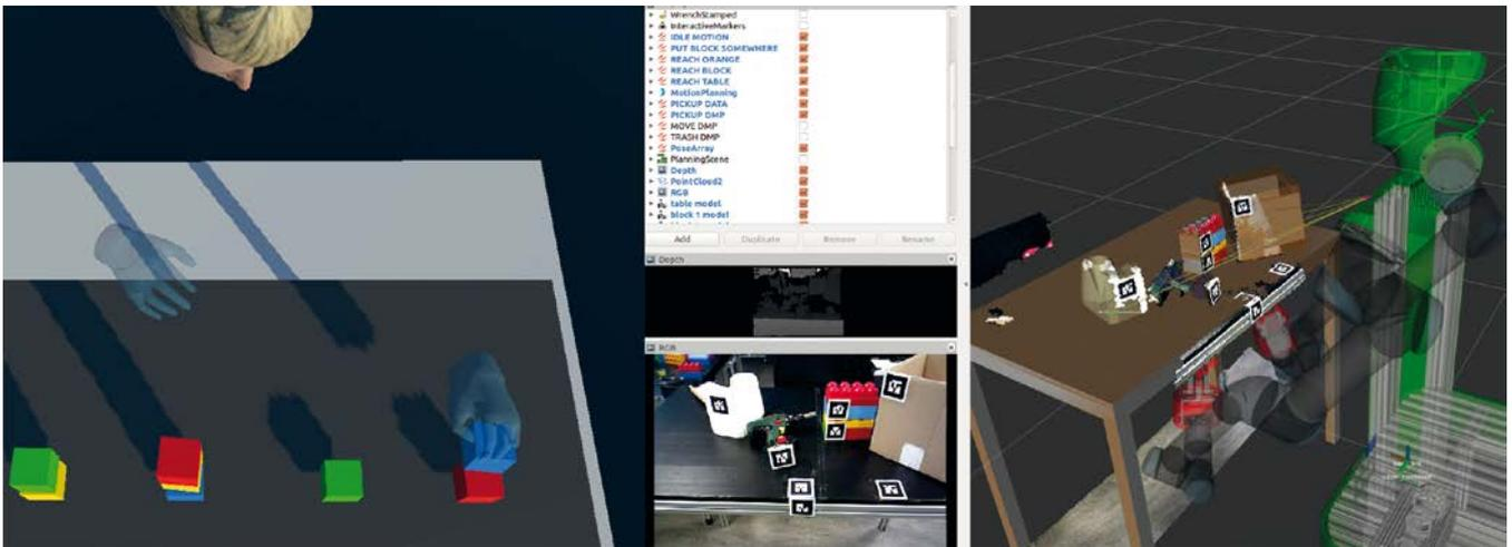
2 | Training using demonstrations of complex tasks performed in virtual reality. Left: virtual reality block-stacking task performed by a human user. Right: instantiation of a complex scene as perceived by the ICS TOM robot.
