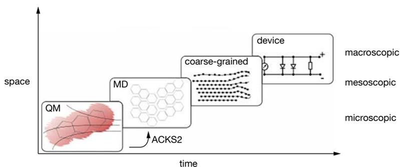
1 | Relevant length and time scales for modeling of charge transport in organic semiconducting materials. The focus of our research group is to bridge the electronic with the molecular scale by developing a novel force field based on the atom-condensed Kohn-Sham density functional theory approximated to second-order (ACKS2) approach.
