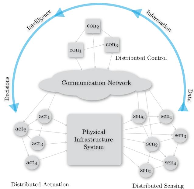
1 | A schematic view of a networked cyber-physical system.
