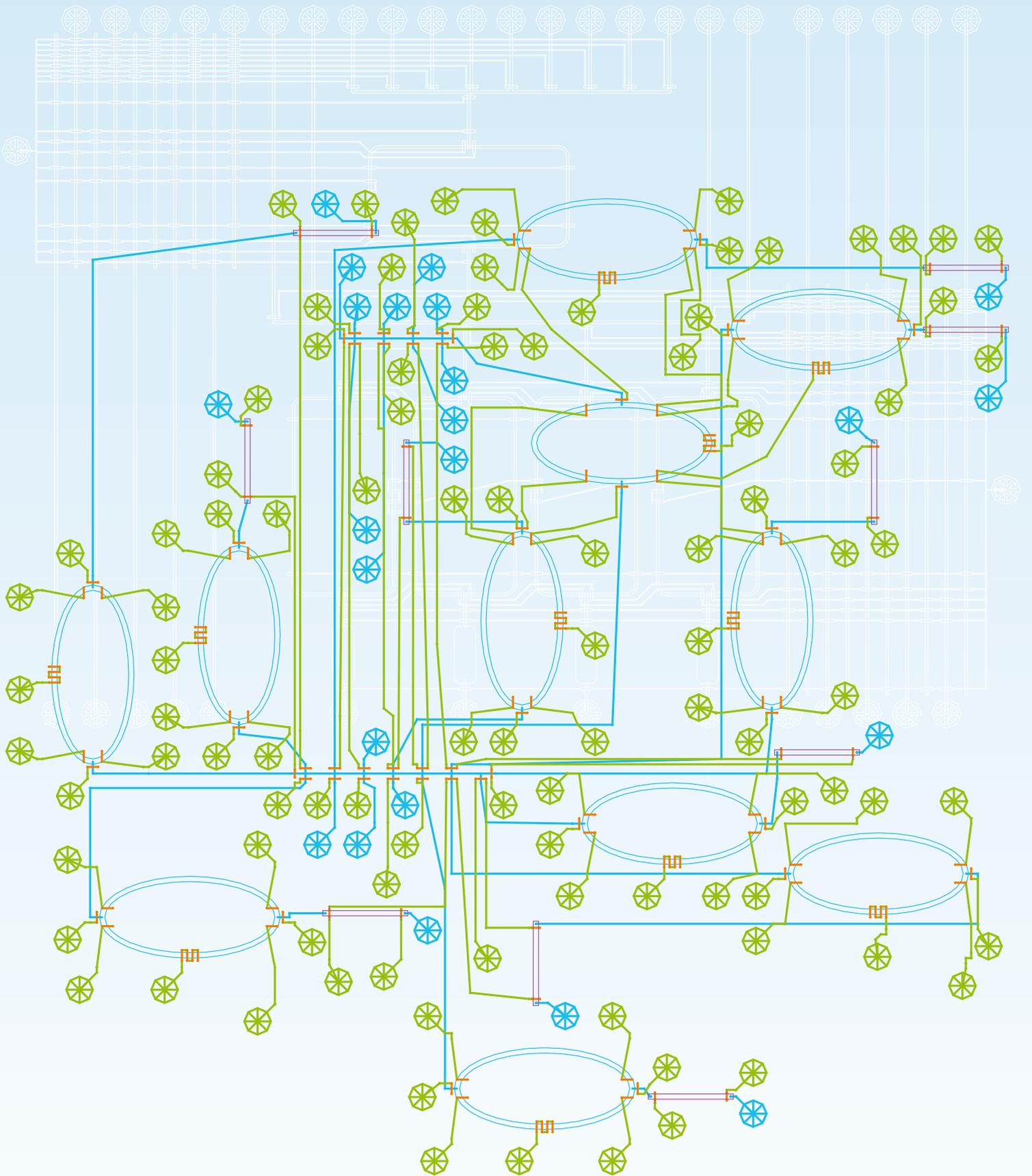
Microfluidic biochip layout from Columba automated design tool.
