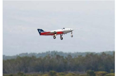
2 | SAGITTA on final approach (left) and just after touchdown (right) within its fully automatic landing on the first flight mission.
