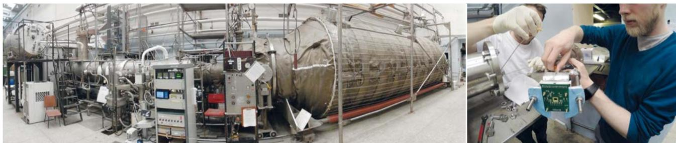
1 | (left) The Troitsk nu-mass experiment in Russia, where the Focus Group characterized detectors for the TRISTAN project. Electrons from the gaseous tritium source on the left are guided by a magnetic field through the large vacuum tank on the right, which houses an electromagnetic filter. Electrons that pass the filter are measured by our detector prototype (right picture), which was installed at the far-right end of the setup.
