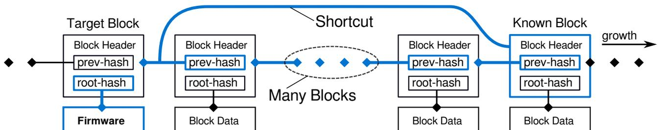
2 | Each new block of a Blockchain stores the hash of the previous block (prev-hash). Verifying the hash of a firmware (stored in a certain target block) requires traversing the blockchain backwards (to the left) block by block. We introduce additional links as a shortcut to reach the target block with fewer intermediate blocks.
