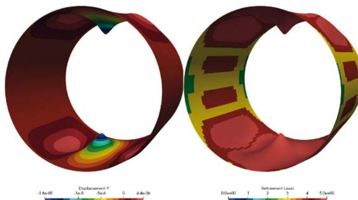
2 | Displacement of a pinched cylinder.
