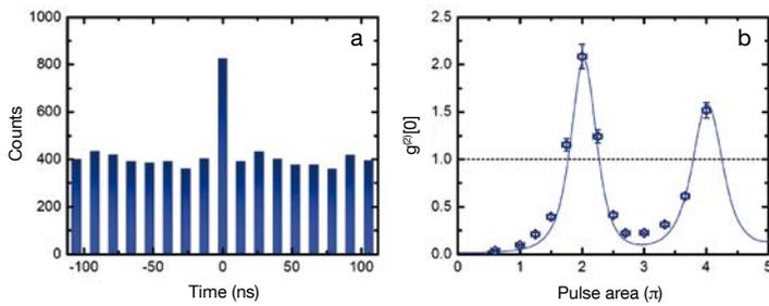
1 |  $g^{(2)}(0)$  as a function of the pulse area for resonantly exciting an artificial atom with short laser pulses.
