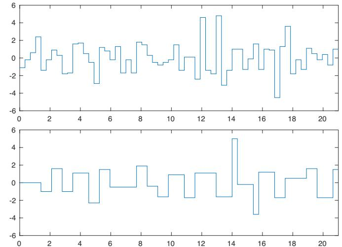
2 | Plots showing the input signal produced by the controller over time. The time intervals where the input signal can be held constant are shown by straight horizontal lines. The upper plot shows the un- optimized controller, while the lower plot shows the optimized controller.
