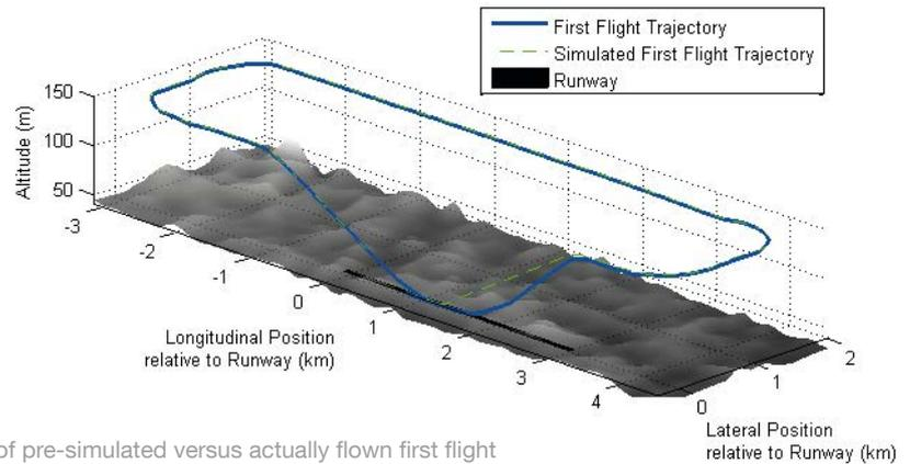
4 | Comparison of pre-simulated versus actually flown first flight mission trajectory of SAGITTA demonstrator.
