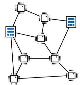
1 | Many existing IoT applications are based on a centralized cloud service. We want to enable a decentralized IoT environment, which establishes efficient communication directly between end devices and results in a more robust infrastructure.
