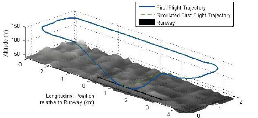
4 | Comparison of pre-simulated versus actually flown first flight mission trajectory of SAGITTA demonstrator.
