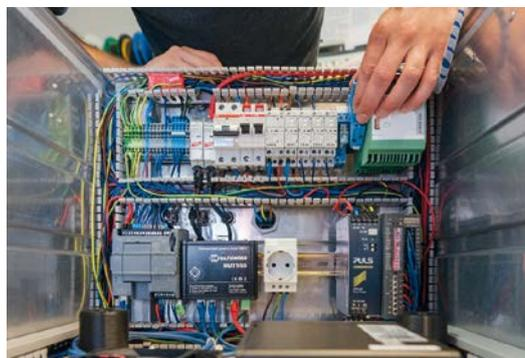
2 | Assembling the enclosure for a spectrometer measuring greenhouse gases
