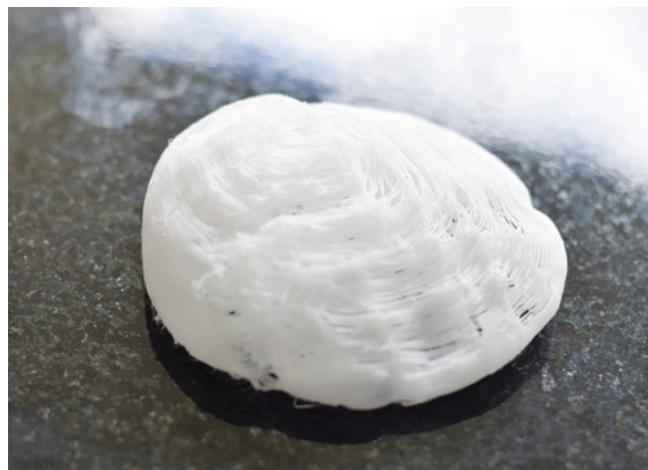
Electrospinning produces a higher resolution of fibers compared to other 3-D printing methods, and results in a network that more closely approximates the structure of natural extracellular matrix. However, state-of-the-art solution electrospinning techniques are not able to control fiber deposition, and the small pore size of the resulting random 2-D meshes ultimately limits 3-D cell migration.
