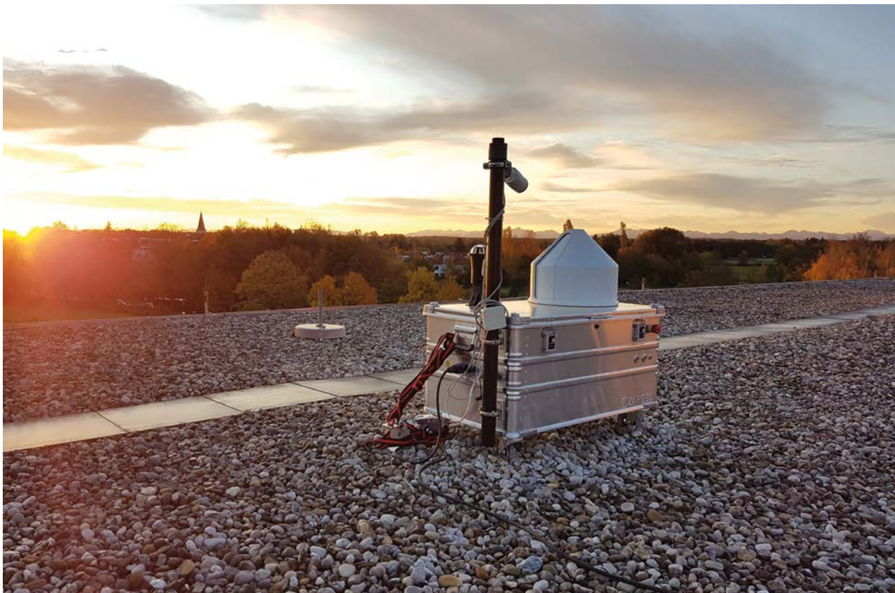
One of the sensors on a TUM rooftop for measuring urban greenhouse gas emissions.
