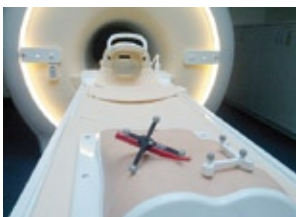
2 | Plastic guiding trokar for the miniature x-ray tube connected to tracking hardware for imaging application with a 3T MRI system.
