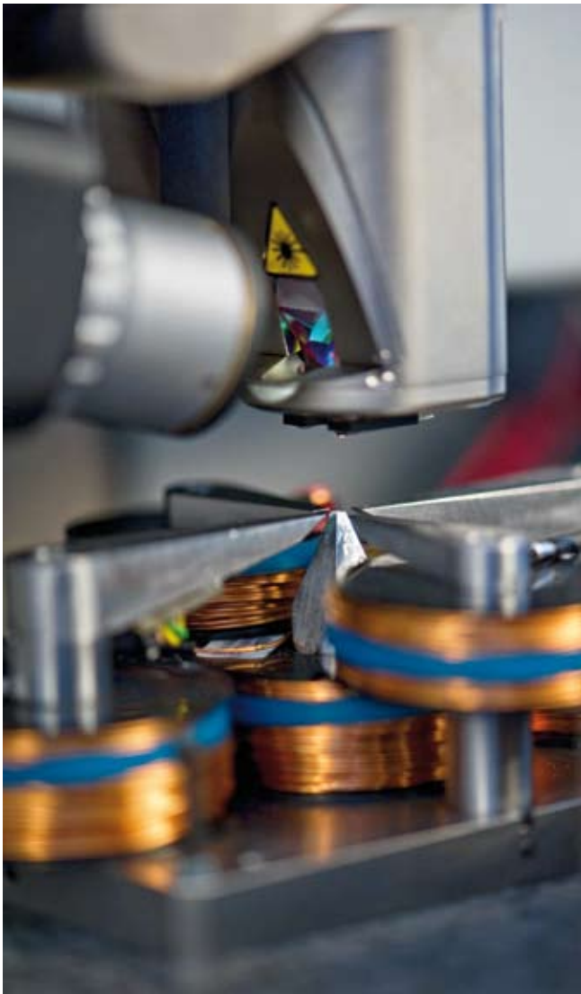
1 | Close-up view of the MFM scanning head above the 3D field-generator.
