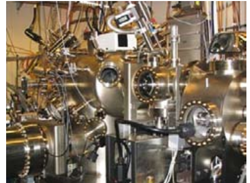
1 | High purity molecular beam epitaxy system for fabrication of semiconductor quantum dots and nanowires
