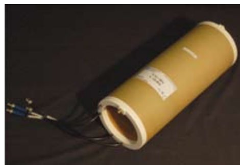
1b | 4-channel ^{13}\text{C} -phased array coil: phased- array coil with housing
