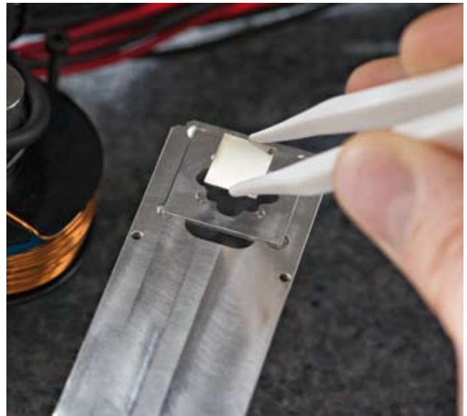
2 | Assembling the microscope with the device under test.
