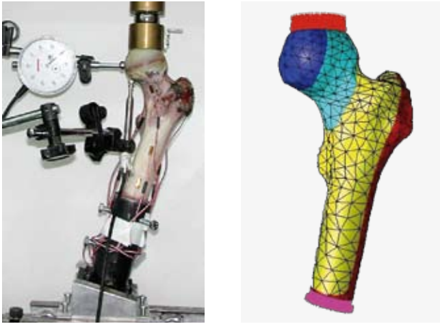
2 | Experiment and high-order-FE analysis of a human femur with displacements prediction.
